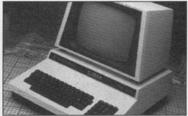
The original PET had a non-standard keyboard, and a built-in screen. The later models had typewriter-style keyboards, with 12" green-on-black screens and a choice of 40 or 80 columns
